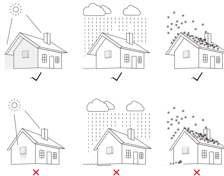
▲ Figure 4.1 Recommended Installation locations
